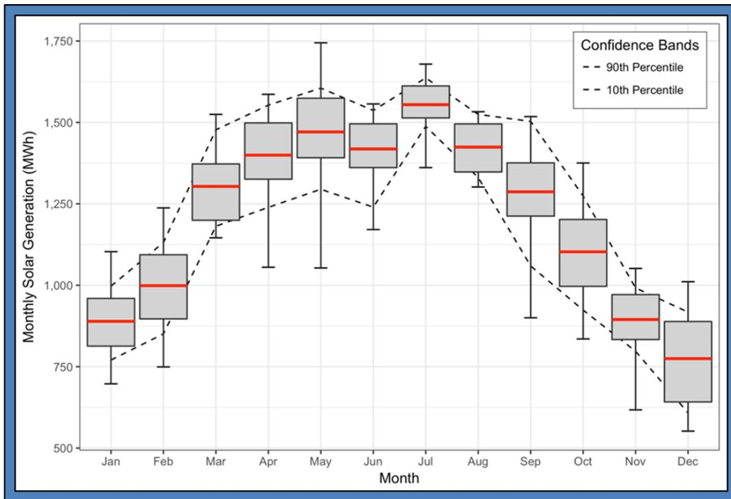
Note: The red horizontal lines indicate the expected value (average), upper and lower box boundaries indicate the P25 and P75 quantiles, and the whiskers extend to the minimum and maximum values of total generation for each month. All statistics are computed over the historical period from 1998 through 2015.
