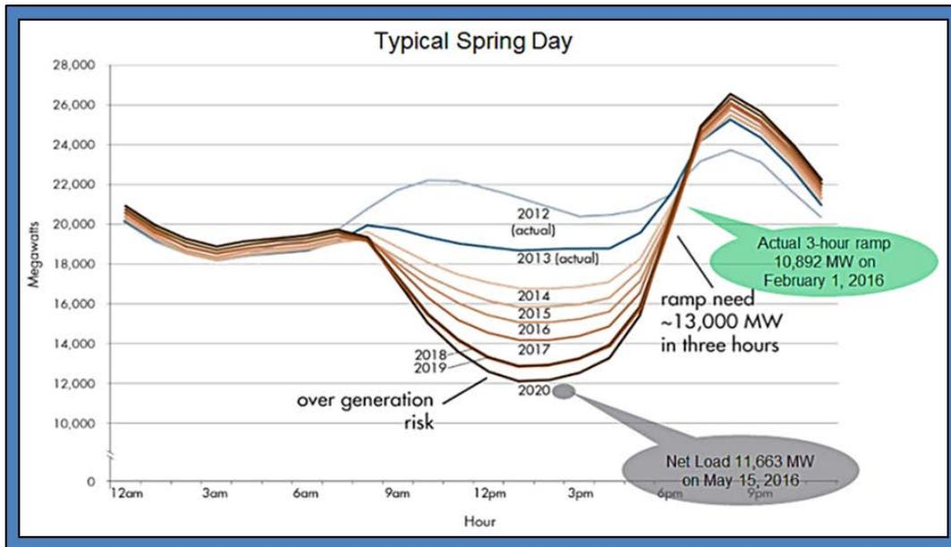
Note: This figure was first popularized in a report by the CAISO in 2013 and has become an iconic representation of how solar generation can significantly reduce mid-day thermal load and exacerbate evening ramping requirements. The reduction in mid-day thermal load can lead to lower (or occasionally negative) marginal prices for real-time electricity.
