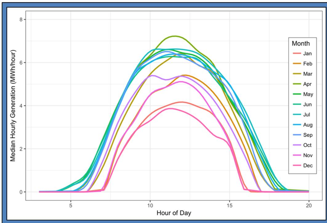
Note: The curves were constructed from 18 years of simulated historical solar generation based on hourly solar irradiance data over the same time period.
