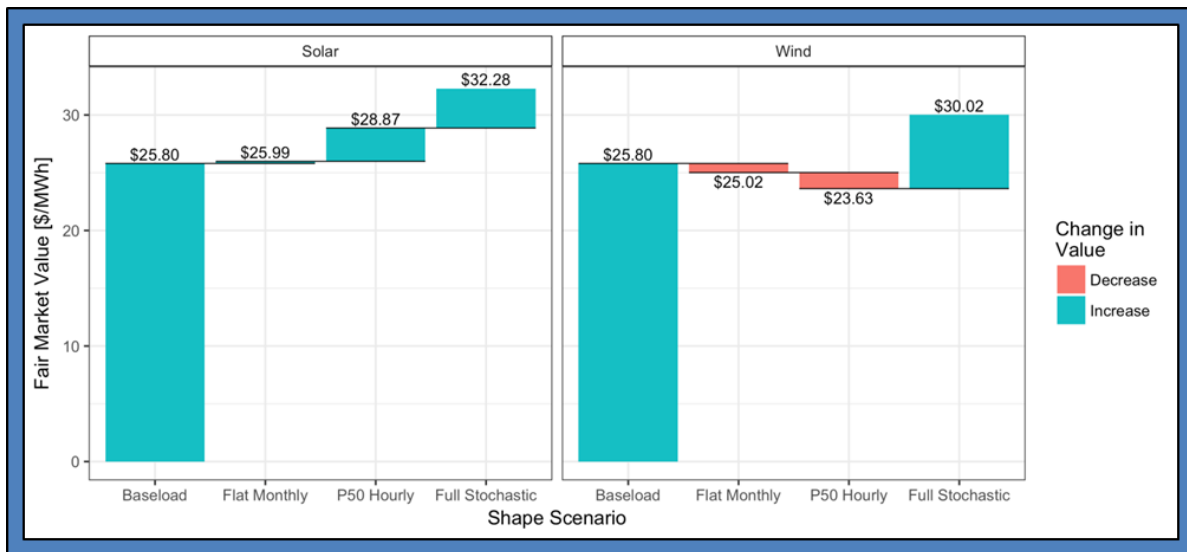
Figure 2 Average Value of Energy Generated for an Example Solar and Wind PPA in Texas under Various Shaping and Valuation Granularities
